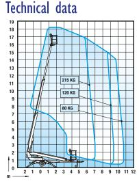
Max. working height 18.00 m Max. platform height 16.00 m Max. outreach 10.70 m Support width 3.8 /4.2 m Lifting capacity 215 kg Basket size 0.70 x 1.30 m Boom rotation cont. Basket rotation 90° Boom control proport. Transport length 7.41 m Transport width 1.78 m Transport height 2.14 m Weight 1840 kg Driving system std AC-socket std Electro motor std Petrol power pack opt. Gradeability 25%
