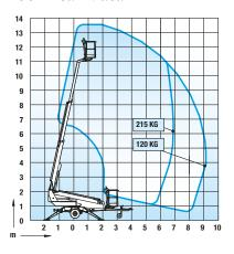
Max. working height 13.50 m Max. platform height 11.50 m Max. outreach 9.10 m Support width 3.8 /4.2 m Lifting capacity 215 kg 0.70 x 1.30 m Basket size Boom rotation cont. Basket rotation Boom control proport. Transport length 5.94 m Transport width 1.78 m Transport height 2.14 m Weight 1635 kg Driving system std AC-socket std Electro motor std Petrol power pack opt. Gradeability 25%
