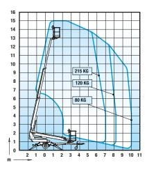
Max. working height 15.00 m Max. platform height 13.00 m Max. outreach 10.00 m Support width 3.8 /4.2 m Lifting capacity 215 kg Basket size 0.70 x 1.30 m cont. Boom rotation 90° Basket rotation Boom control proport. Transport length 6.43 m Transport width 1.78 m Transport height 2.14 m 1670 kg Weight Driving system std AC-socket std Electro motor std Petrol power pack opt. Gradeability 25%
