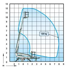
Max. working height 12.00 m Max. platform height 10.00 m Max. outreach 7.90 m Support width 3.15/3.55 m Lifting capacity 120 kg Basket size (round) ø 0.85 m Boom rotation cont. Boom control 2-speed Transport length 5.52 m Transport width 1.72 m Transport height 1.96 m Weight 1285 kg Driving system std AC-socket std in the basket x 2 Electro motor std Petrol power pack opt. Gradeability 25%
